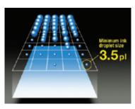
The PrecisionCore technology, as well as Variable Size Dot Technology, allow the ink droplets to be controlled to the finesse of 3.5 picolitres.
